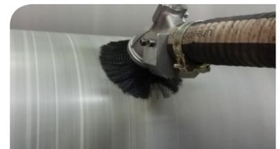
Surface regeneration is needed in order to get back an appropriate surface roughness
